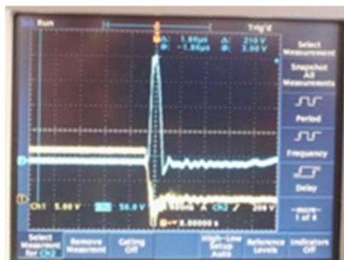
Fig. 2. The oscilloscope image showing the pulse generated by the pyroelectric device in the QB; Here, pulse height = 210 V, pulse width = 100 nsec, and frequency = 10 MHz.
