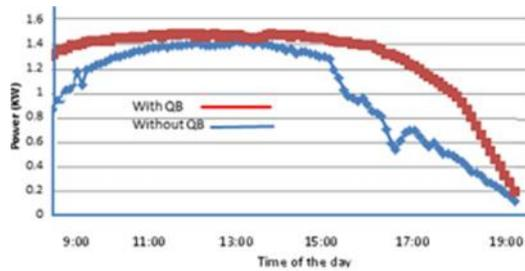
Fig. 4. Power output from a solar cell panel string with and without the QB measured on two different days having similar light conditions.
