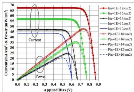
Fig. 6. The simulated  $I - V$  and  $P - V$  characteristics of solar cells as a function of QB-generated electron collection in a typical solar cell by high frequency and high voltage pulses.
