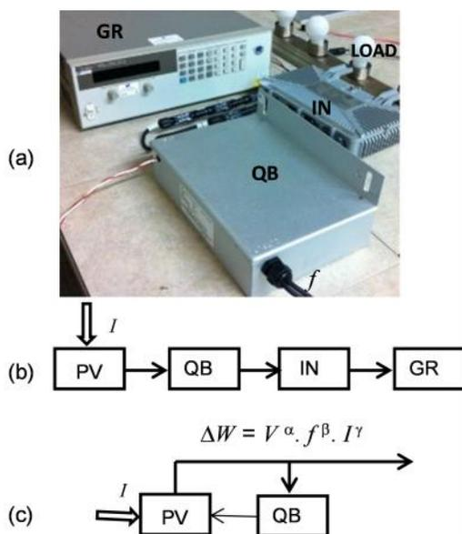
Fig. 1. Measurement system: (a) photograph; (b) Schematic diagram of the test configuration showing photovoltaic panel (PV), Quantum Boost (QB), Inverter (IN), and Grid Simulator (GR); where  $I$  is the intensity of incident solar radiation; (c) increase in the power output of the PV by high voltage ( $V$ ) and high frequency ( $f$ ) pulses.
