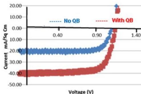
Fig. 3.  $I - V$  curve of a silicon solar cell under 0.44 sun intensity with and without the QB.
